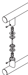
Adapterset zur beidseitigen Montage Holztüren Adapter set for bilateral installation, wooden doors
